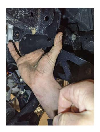
Install the rear brackets as shown here using supplied bolts, spacers, and lock nuts. Reinstall the upper and lower shock bolts using original hardware.
