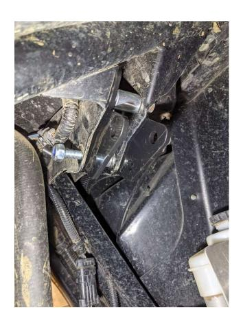
Install the front brackets as shown here using supplied bolts, spacers, and lock nuts. Notice how the wire that runs here must be removed from its mounting in order to clear the new bracket. Reinstall the upper and lower shock bolts using original hardware.
