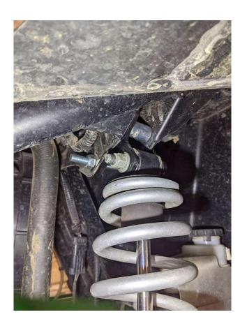
Make sure that all bolts are tight (refer to factory specs). The front bracket has two shock locations – the outer one is for a leveled look, the inner one will retain a slight "rake" to the front end like factory (sits slightly lower in front). If you would like additional lift, crank the settings up on the shock adjusters.
