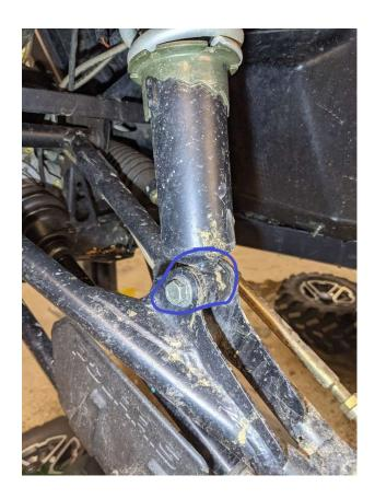
Lift vehicle, remove wheels, then remove upper and lower shock mounting bolts as circled in pictures here:
