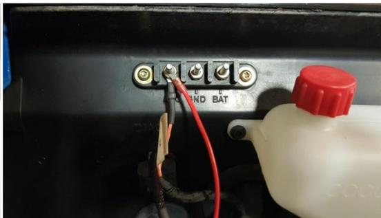
16. Verify operation of Horn. Turn Key on and the Bottom Switch LED should illuminate, Push the top of the Horn Rocker and the Horn should sound.
