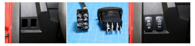
**Dielectric Grease**- Just like the OEM uses on their switches, we recommend using Dielectric Grease on all switch terminals, this keeps the water out, thereby reducing corrosion and helps increase reliability! Open the grease and put on the switch terminals and the connector terminals on both the Turn and Horn/Hazard switches, the more the better.
