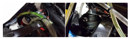
9. Run power wire to 12vdc accessory stud under the hood and ground the black wire.
