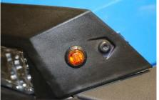
Run the short front harness through rubber grommet to the front right LED. Connect the green wire to the black and the white to white, continue harness to left LED, yellow wire attaches to black wire and the white wire goes to white. NOTE: Black wire is positive and will not work if reversed. White is ground. Secure the Harness using the provided cable ties.
