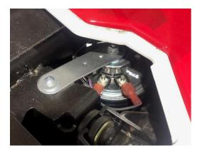
8. Plug the Power Harness into the Control Module. Run the power wire to the Busbar, remove one of the blanks and plug into the Busbar. Use one of the provided screws to secure the fuse holder.
