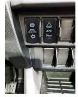
Run Switch Harness—Plug the Switch Harness into the Control Module, run the two connectors through the rectangle switch cutouts and use included grease (see above) then connect to turn switch and slide switch into dash. **NOTE:** The switch cut outs are counter sunk, we have supplied 4 switch seals (2 for each Switch) to be used as spacers to keep it raised out of the indent to keep it from getting stuck.
