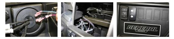
8. **Dielectric Grease** - Just like the OEM uses on their switches, we recommend using Dielectric Grease on all switch terminals, this keeps the water out, thereby reducing corrosion and helps increase reliability! Open the grease and put on the switch terminals and the connector terminals on both the Turn and Horn switches, the more the better.
