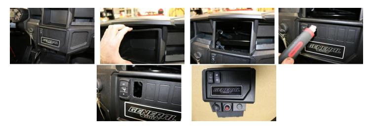
7. Run Switch Harness - Push the 10 pin Horn connector through the grommet in center, then push the 8-pin Turn switch connector through. Note: The grommet can be removed and stretched over the switch connector and reinstalled. Run the connectors through the rectangle switch cutouts and use included grease (see step 9) then connect to turn switch and slide switch into dash as shown.
