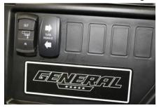
**Dielectric Grease** - Just like the OEM we recommend using Dielectric Grease on all switch terminals, this keeps the water out and will also reduce corrosion and increases reliability! Open the grease and put on the switch terminals and the connector terminals, the more the better, also put on the Horn/Hazard switch terminals. It should also be used on any extra switches that you may have installed.
