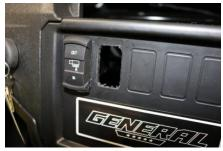
7. Run Switch Harness – Plug the Switch Harness into the Control Module, run the two connectors through the rectangle switch cutouts and use included grease (see step 9) then connect to turn switch and slide switch into dash.
