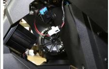
12. Re-install the Kick Panel. Verify operation of all lights. Cable tie any extra harness under dash.
