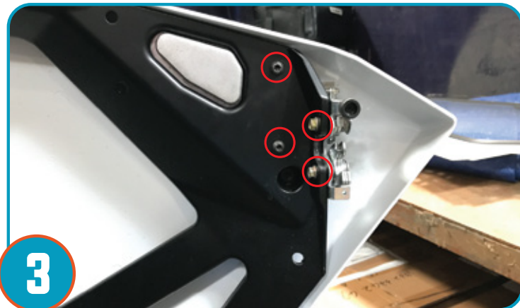
Remove four bolts holding OEM Paddle latch on the stock door. Repeat for opposite door.
