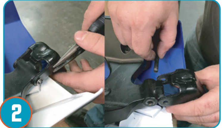
Stock hinges will be used for your Pro Armor door. Remove hinge by carefully removing the clip and sliding the pin from the hinge. Remove hinge from stock door. Remove bushings from door. Repeat for opposite door.
