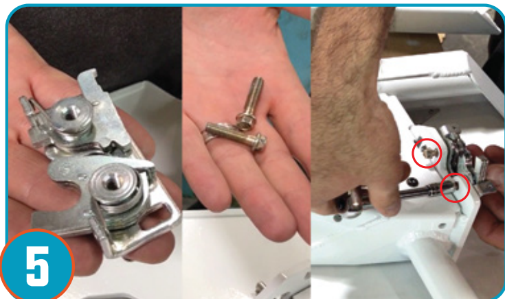
Using the provided bolts, secure the latch to latch plate as shown. Repeat for opposite door.
