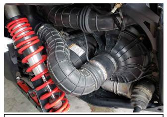
Slide the Blow Hole over the clutch cover. Install clutch intake tube back onto stock intake duct. Tighten all clamps. Make sure the clutch intake tube is not touching the shock spring.
