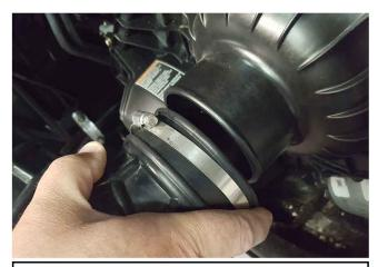
Remove the clutch intake tube by loosening the clamps on both ends of the clutch intake hose.
