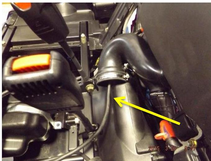
4. Pull excess wire out of the exhaust hose to allow for easy install of blow hole.
