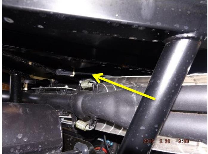
5. Route wiring harness to the driver side of the RZR so you can plug into the tail light harness. Ensure wiring is routed over the support bars to prevent any heating or damage to the wiring.
