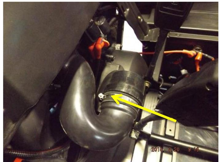
7. Connect silicone end of blow hole to the clutch housing and tighten clamp. Ensure the clamps are as shown to prevent the engine access panel from pushing the clamps into the hose.
