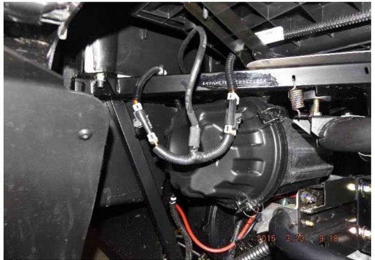
9. Secure wiring to ensure no damage occurs while the RZR is in use. This will also prevent any part of the wiring harness from being exposed to engine components.
