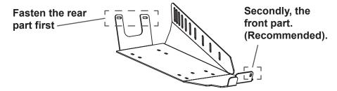
Using a riveting tool, place the rivets on the bottom part of the RockSlider in the holes provided. Use a washer for each rivet (Included). Recommended: First place the 2 rivets of the front holes, (Fig. 1), and then, place 2 rivets on the rear holes (Fig. 2). This will help to have an easier installation on the remaining rivets.
