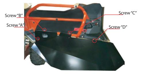
Remove the rivets from the handle guard on the inside of the door. Remove the handle guard and the plastic on the structure of the upper door.
