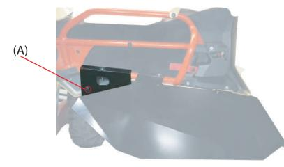
Line the half lower door with the original holes from the upper door structure (tube). Starting from A to D.
