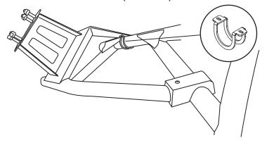
Finish by aligning the Spare Tire Carrier and then tighten the bolts.
