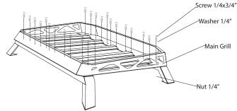
Please assemble the Roof Rack (completely set) over the roof, aligning it with the perforations done in the first step. Use 4 1/4 x1" screws with the washer and nut.
