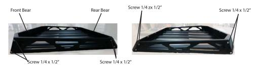
Set the Front and Rear legs (as it is shown in the image) using 8 1/4x1/2" screws with nuts.
