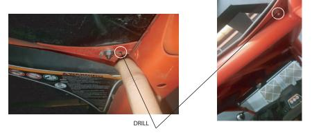
Place the Front and Rear corners with the lateral (as it is shown in the image). Use 8 1/4 x 1/2" screw with nuts.
