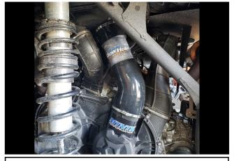
Install the Blow Hole by slipping the silicone over the clutch cover intake duct first and then slide the top silicone over the upper duct. Once installed, tighten stock clamps as shown.
