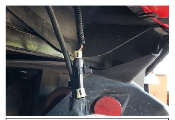
Locate the factory tail light connector and plug Blow Hole directly into the tail light as shown.
