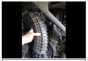
Remove the clutch intake tube by loosening the clamps on both ends of the clutch intake hose. This clutch intake tube will not be used. Keep the clamps for later use.
