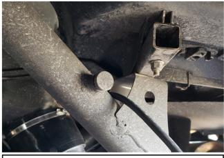
Route the wiring harness over the cage as shown and proceed to route wire up towards the tail lights. Be sure to route wire so it does not rub or chafe. Use wire ties if needed.
