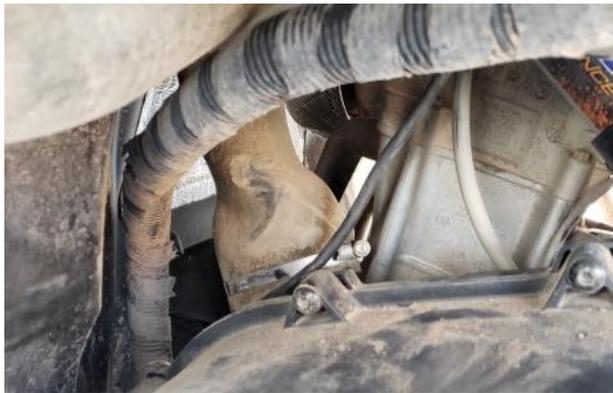
3. Carefully Route the Blow Hole wiring harness down the factory harness and under the driver seat towards the front of the machine. Secure wires so they do not rub.
