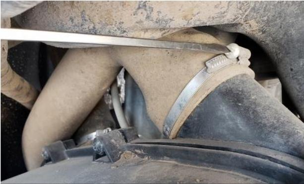
1. Remove Driver's seat. Locate rubber duct located on top of the clutch cover. Loosen hose clamp and remove rubber duct. You will re-use the hose clamp.
