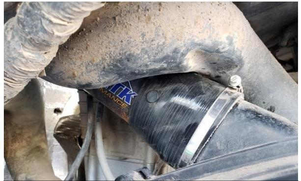
2. Install Blow Hole as shown onto the clutch cover with straight silicone towards the clutch cover. Align MTNTK Graphics as shown. This will insure proper routing. Use the stock clamp and fasten the Blow Hole to the Clutch Cover.
