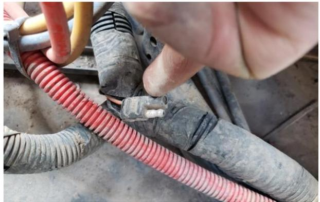
4. Locate the stock accessory plug and insert the Blow Hole harness plug: Red to Orange, Black to White. This allows you to still use the factory accessory plug. Reinstall Driver's seat.
