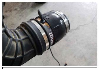
Install the Blow Hole inside the clutch intake tube by heating up the tube and stretching it over the Blow Hole. Make sure the wire is pointed upward as shown.
