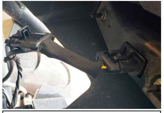
Locate the factory tail light connector and plug Blow Hole directly into the tail light as shown. Route wire so it does not rub or chafe.
