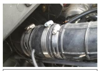
2. Install the Blow Hole onto the Clutch housing as shown. Tighten clamp. Then install the intake duct hose onto the Blow Hole assembly. Tighten clamp.
