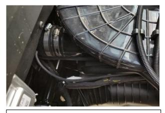
1. Locate the clutch housing intake duct hose. Loosen the clamps holding it onto the clutch cover and remove hose from housing.
