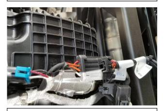
3. Unplug tail light connector and plug in Blow Hole connector in line. Properly route and secure wires and connectors with cable ties as needed to prevent damage.
