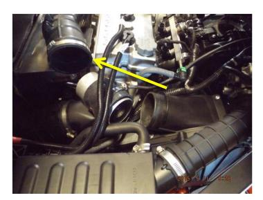
4. Now install Blow Hole onto Clutch housing as shown. Tighten clamp.
