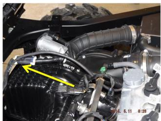
8. Check vent to ensure blow hole is forcing air out and not in.
