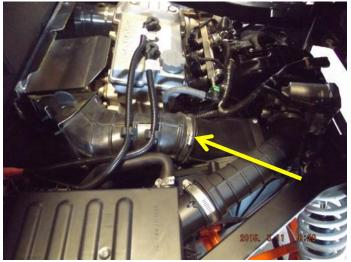
3. Separate the exhaust hose from the Clutch Housing.
