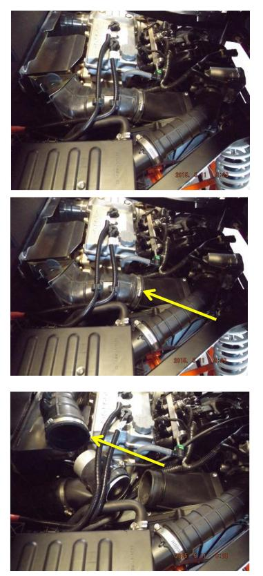
3. Separate the exhaust hose from the Clutch Housing.
