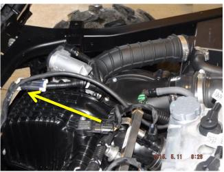
8. Check vent to ensure blow hole is forcing air out and not in.
