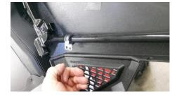
Step 2: Install U clamps (front and rear) by adjusting the center hole of the panel on original door center hole. Then remove panel and place the U-nuts so that the tube clamps are held in the correct position, aligning the holes
