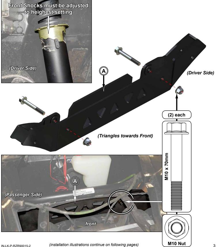
Rear Installation: Do not tighten hardware completely until last step. Keep all components removed.
