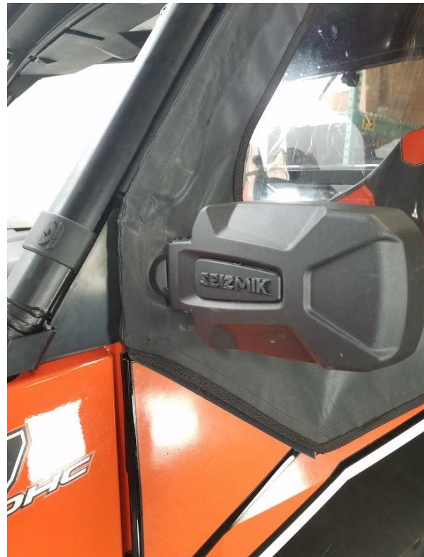
18. Pass the bolt through the mounting bracket and thread into the mirror and tighten (DO NOT OVER TIGHTEN).
