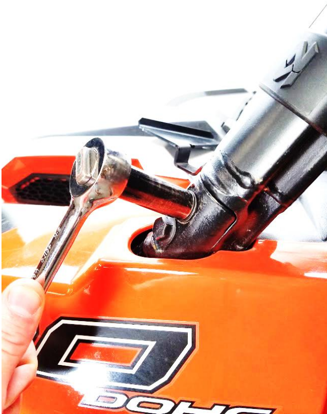
11. Remove the factory roll cage bolts.
