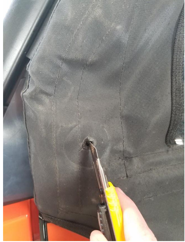
17. Using a sharp razor or utility knife, cut the textile so the mirror mounting bolt can pass through.
