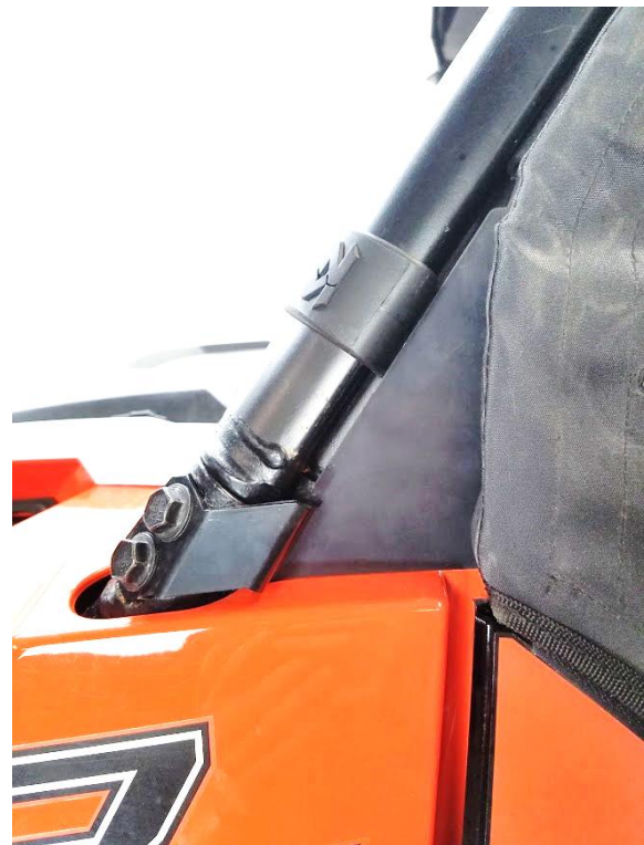
13. Re-Torque the Factory Cage bolts to Polaris Spec's.
