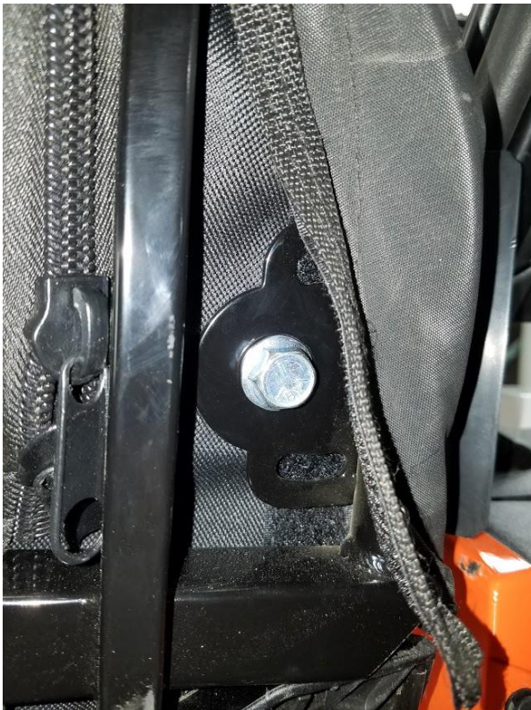
18. Pass the bolt through the mounting bracket and thread into the mirror and tighten (DO NOT OVER TIGHTEN).
