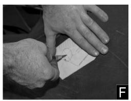
**Step 8:** Center the drill and then drill a 1-1/8" hole on the plastic of vehicle. (Figure G)
