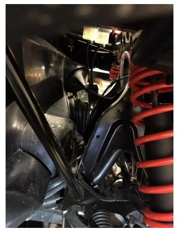
Take the heater box and place it in the position it will be mounted (see below). Mark the mounting holes and pre-drill with a 1/8" drill bit. Also, mark the spot on the firewall where the heater hose will run to the front of the machine, this spot will be straight off of the inlet/outlet fittings from the heater box (see picture above). Now take a 1 ½" hole-saw and drill through the firewall, this is where you will run the two heater hoses to the front of the machine.
