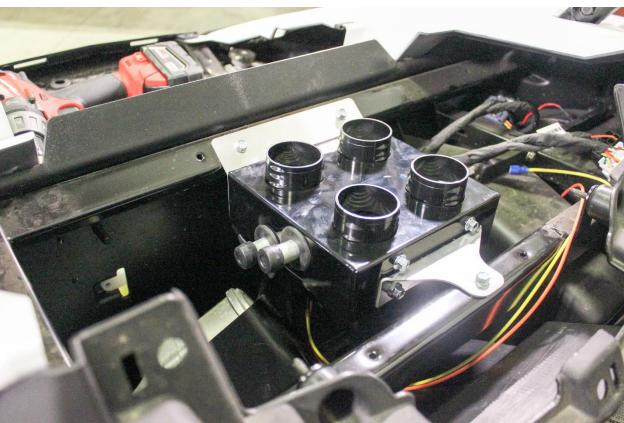
Now install the rubber grommets into the firewall. Use a 1 3/8" hole-saw to make the two holes, then install the grommets. Cut 4-foot piece of hose and connect it to the higher heater core fitting (relative to gravity); install the remaining 3-foot piece on the lower heater core fitting (relative to gravity). Run the hose through these grommets and into the front of the machine and leave them until you install the Y-fittings.
