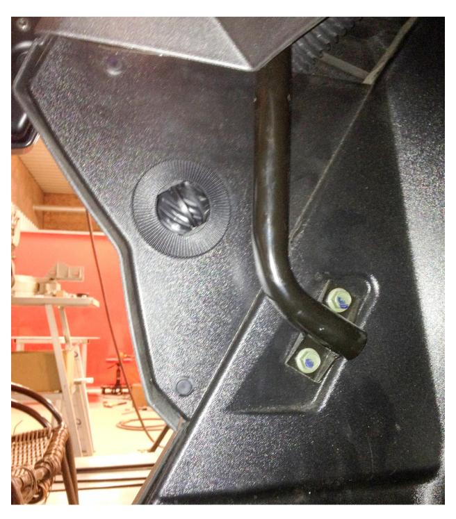
Last, attach the duct hose to the louvers and secure with the zip ties provided. Make sure you use a needle nose pliers and bear down on the zip-tie to insure a tight hold. Then run the hose up to the heater and secure with a zip tie to the heater box duct adapters. After all four louvers are attached you can reattach your dash panel and fenders.
